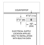
NOTE: Dimensions in parenthesis are in millimeters unless otherwise specified
