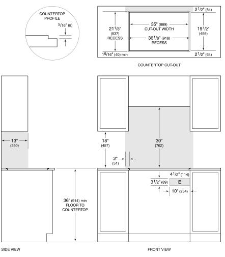
NOTE: Shaded area above countertop indicates minimum clearance to combustible surfaces, combustible materials cannot be located within this area. Electrical supply location only applies to installations with built-in oven. Outside corner radius 7/16" (11).
